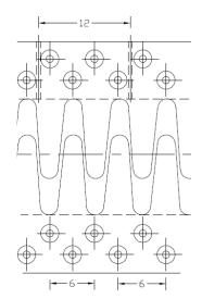
Ply-Seal® Joint System with 2" Removable Finger Plates
